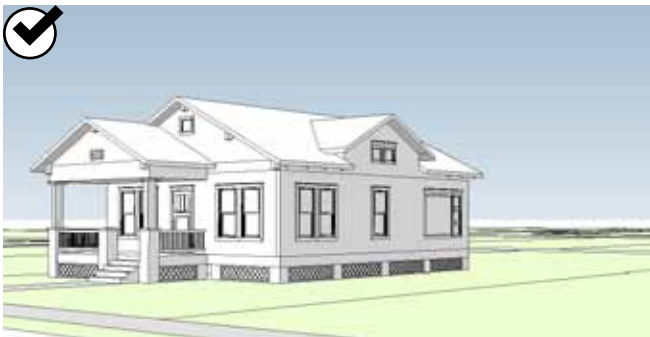
3. Side addition with gable roof
