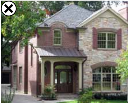
The mass and scale of this infill building would be appropriate. However, the stone materials, shutters, and solid-to-void ratio are incompatible.
